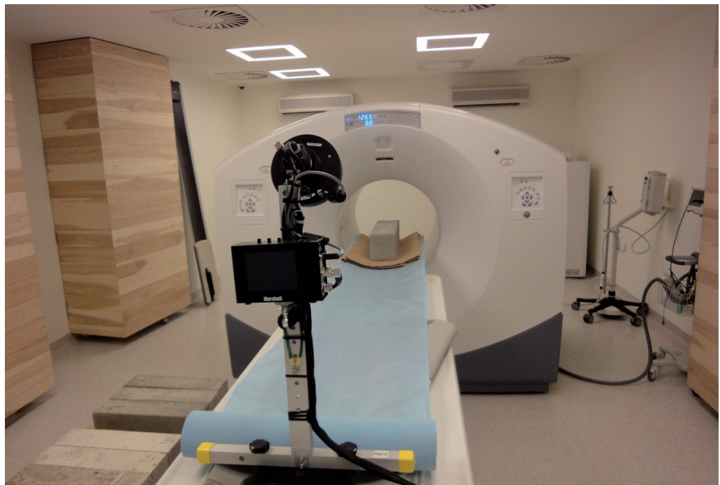
Fig. 4. The CT scanner equipped with 64 rows of detectors
