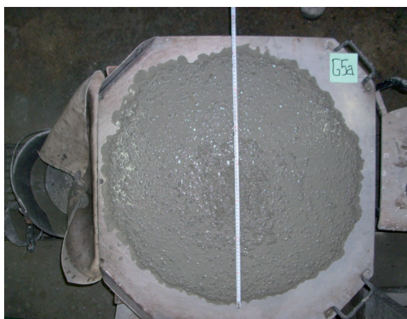
Fig. 2. Slump-flow test and SFRHPSCC beams C4 600x150x150 mm
